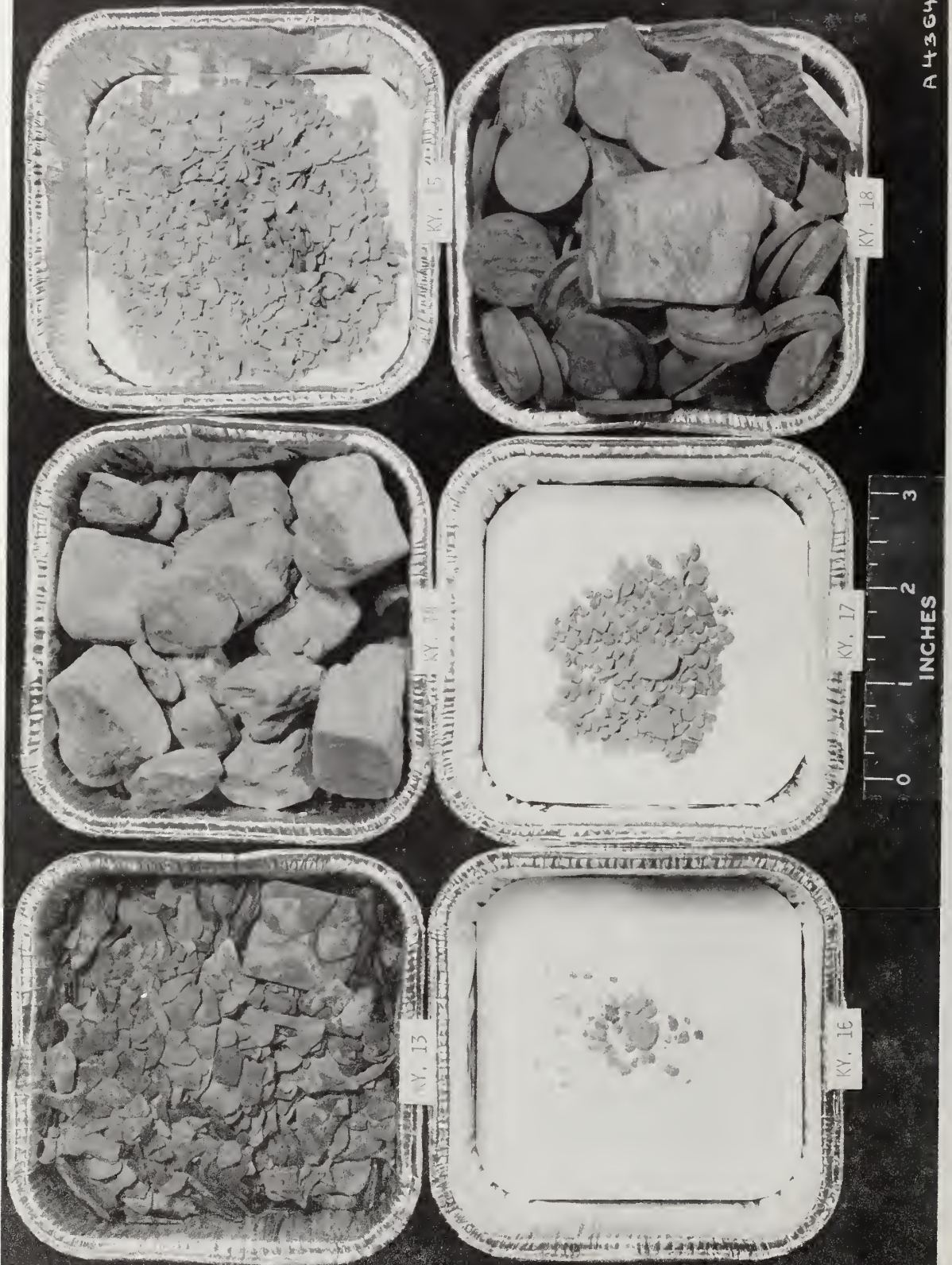
Figure 39. Material remaining after slake-durability testing, KY 13-KY 18.
